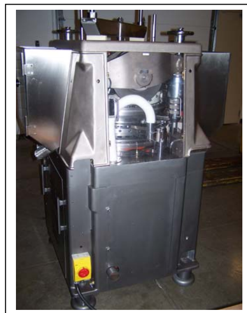
MKII VFD Retrofit - Eliminates Lathe Shaft, Variable Speed Pulley, and Clutch Assembly
